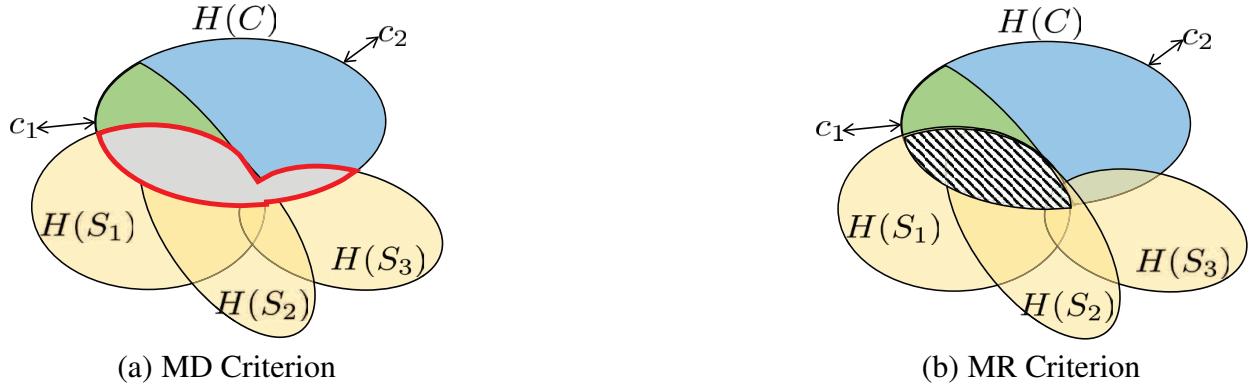
Figure 4.2: Venn Diagrams for Maximum Dependency (MD) and Maximum Relevance (MR) criteria
